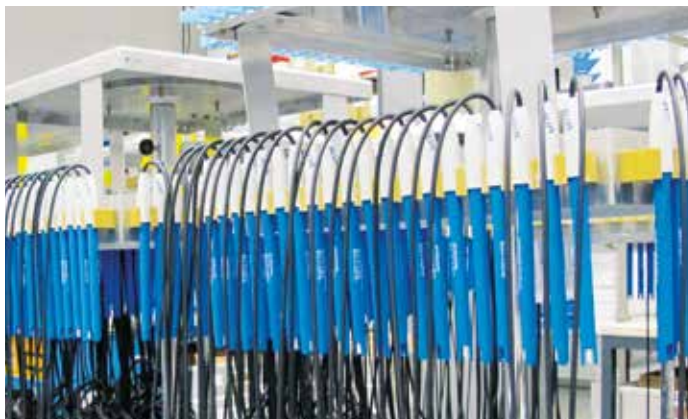
Thorough quality control is an essential element from start to finish. The zero point and response time of every electrode is checked – as shown here with a batch of BlueLine laboratory electrodes.
