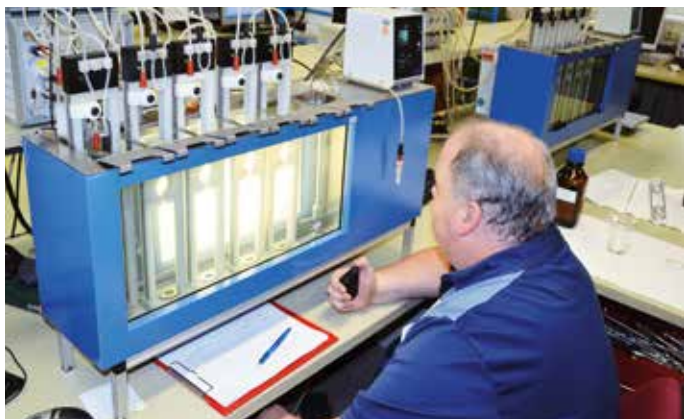
With the processed calibration, the viscometers are provided with an ID number and a certificate documenting the specific characteristics.
