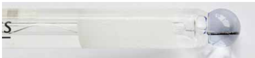
③ Blue pH glass ball at the tip of a pH electrode.
