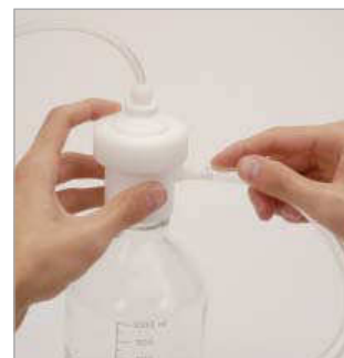
Connect vacuum line to side port.
