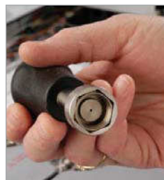
Septum nut remains in tool until reinstalled.
