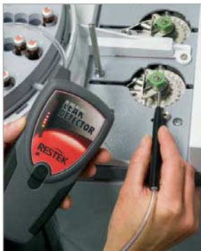
Checking for leaks maintains the integrity of a GC system.
