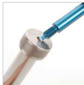
Insert the tool into the center hole of the extraction cell cap.
