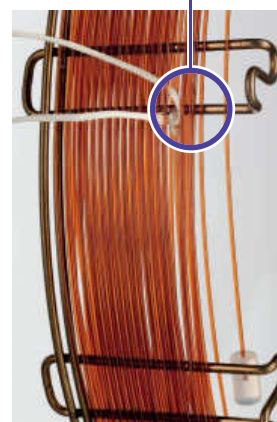
String indicates where the analytical column begins.
