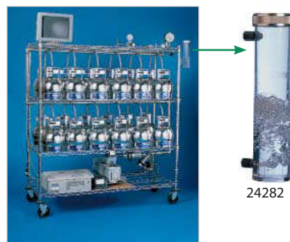
Restek's canister cleaning system with humidification chamber.
