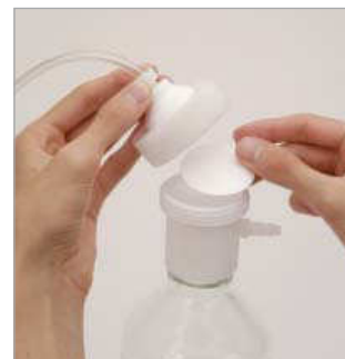
Place membrane filter on top of grid.
