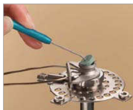
Remove a septum without damaging an expensive weldment.
