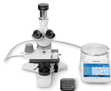
Microscope equipped with Hot-Stage 84
