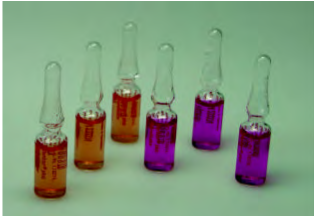
Figure: Sterikon® plus bioindicator for steam sterilization (121°C for 15min.)
