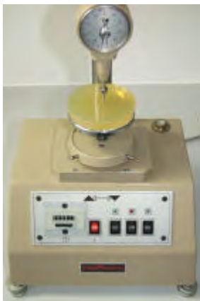
Figure: Measurement of gel strength with Costin's Gelomat
