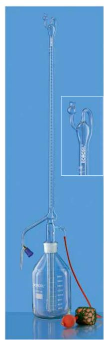
Automatic Zero, Accuracy as per Class A of IS 1997:2008/EN ISO 385, with Reservoir, Rubber Bellow and Boroflo Stopcock, With Certificate
