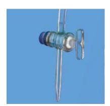
Automatic Zero, Accuracy as per Class A of IS 1997:2008/EN ISO 385, with Reservoir, Rubber Bellow, Glass Stopcock, Amber With Certificate
