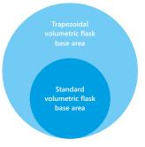
Volumetric flasks with small capacities can be topple down more easily due to their higher centre of gravity.
