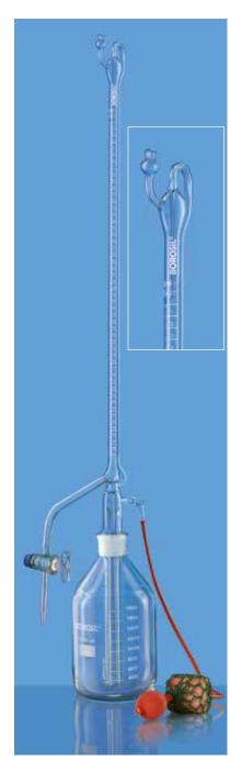
Automatic Zero, Accuracy as per Class A of IS 1997:2008/EN ISO 385, with Reservoir, Rubber Bellow, Glass Stopcock, With Certificate
