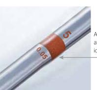
All pipettes are colour coded at the top to allow fast identification
