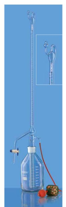
Automatic Zero, Accuracy as per Class A of IS 1997:2008/EN ISO 385, with Reservoir, Rubber Bellow, PTFE Stopcock, with Certificate
