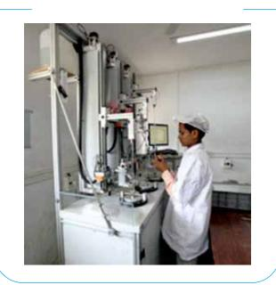
Computer controlled automatic calibration machine with optical laser beams to prevent human error and ensure highest level of accuracy and precision
