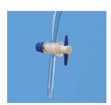
Automatic Zero, Accuracy as per Class A of IS 1997: 2008/EN ISO 385, with Reservoir, Rubber Bellow, PTFE Stopcock, Amber With Certificate
