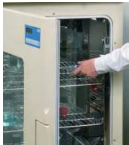
Optimum temperature homogenization can be achieved with an even load distribution of up to 70% unit volume.
