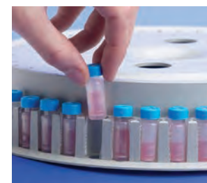
Whatman Mini-UniPrep in an HPLC autosampler
