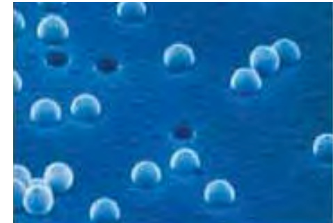
Electron micrograph of Cyclopore membrane with latex beads on surface
