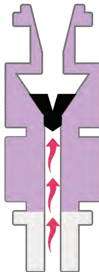
The membrane is a barrier against eluent vapours and gas leaks.
