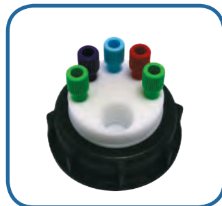
SW55-5-C : 5 entries 1/8" and a charcoal cartridge emplacement
