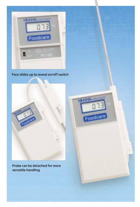
**SPECIFICATIONS** HI 149-00 HI 149-01 Range -40 to 300°C -40 to 572°F Resolution 1°C 1°F Accuracy ±2°C ±4°F interchangeable, stainless steel probe with 1 m cable (not included) Probe Battery Type / Life 1.5V (3) / approximately 700 hours of continuous use 0 to 50°C (32 to 122°F); RH max 95% Environment **Dimensions** 106 x 68 x 21 mm (4.2 x 2.7 x 0.8) Weight 80 g (2.8 oz.)
