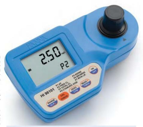
This multiparameter photometer can save time and money. If you need a simple, but professional meter measuring the most important constituents of water, especially in pools and spas, then HI 96101 has been designed for you.
