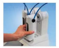
contamination while reducing loss of time and reagents. Burettes simply slide out for quick exchanges and detaching the aspiration and dispensing tubes from the titrant bottles is easy.
