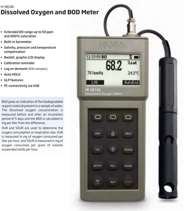
HI 98186 portable Dissolved Oxygen Meter has extended ranges of up to 50 ppm or 600% saturation. This instrument includes barometric pressure measurement and calibration with a user selectable unit (mmHq, atm, mbar, psi, kPa) as well as a 1 or 2 point temperature calibration. Salinity, pressure and temperature compensations enhance the precision of your readings.
