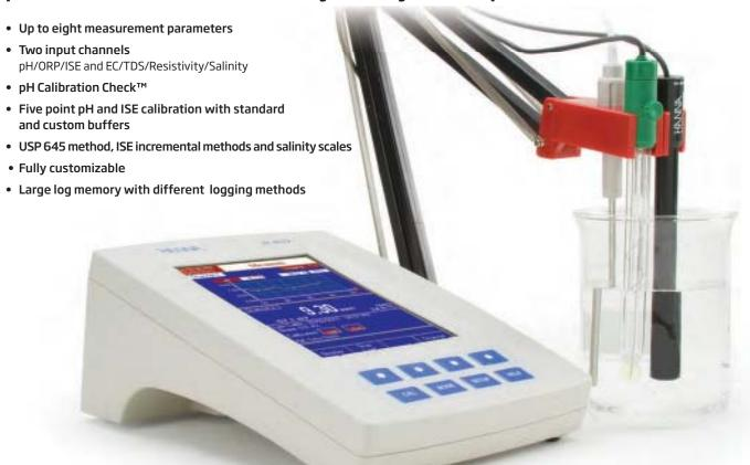
HI 4521 and HI 4522 are research grade, benchtop instruments that feature 8 measurement parameters: pH, ORP (Oxidation Reduction Potential), ISE (HI 4522 only), conductivity, resistivity, TDS, salinity and temperature. These instruments incorporate dual channels with a separate temperature input and support the external reference electrodes required by half cell pH and ISE sensors.
