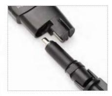
Replaceable pH electrode cartridge
