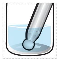
hydrate a dehydrated glass sensor, thoroughly wetting a dried reference junction (wick, ceramic etc).
