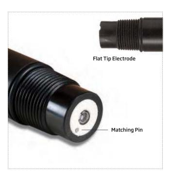
from external electrical fields. Shown above, the matching pin allows the measurement to stabilize and ensures effective process regulation. In order to function properly, the matching pin has to be continuously immersed in the measured solution and for this reason is placed near the electrode junction.
