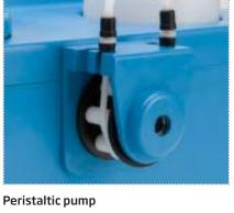
The HI 84430 features a precision peristaltic based titrant delivery system.
