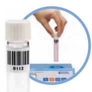
Bar code reader detects the method and range automatically
