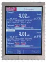
calibration. There are many influences including aging, temperature, coatings, and chemicals used that will affect the characteristic. So the question becomes 'what is a typical probe characteristic and how do you check it?'
