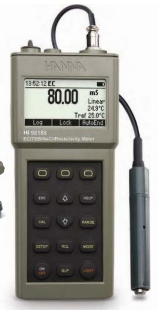
HI 98188 is a waterproof, portable conductivity meter that has an expanded conductivity range from 0.001 µS/cm to 400 mS/cm, as well as TDS, resistivity and three salinity scales. This meter automatically recognizes the probe type (two or four ring) and allows the user to adjust the nominal cell constant. HI 98188 is also ready to perform all three stages of USP <645> method required for EC measurement of pure and ultrapure water.
