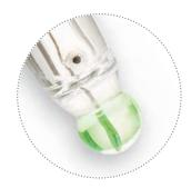
A spherical tip is recommended for general use in aqueous or liquid solutions and provides a wide surface of contact with the sample.
