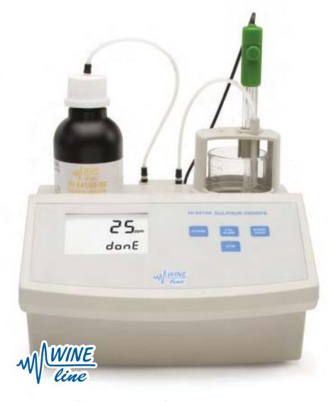
The HI 84100 offers the possibility to test free or total  $SO_2$  in all the wines including the red ones, that are difficult to test with manual methods because the color changes are hardly seen.
