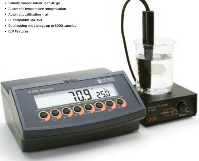
HI 2400 is a dissolved oxygen benchtop meter with automatic calibration and % or mg/L (ppm) measurement range. The measurement is automatically compensated for altitude and salinity compensation based on the user settings for altitude up to 4000 m and 40 g/L for salinity.
