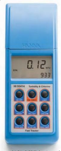
With the powerful CAL CHECK™ function, performance of the instrument can be validated at any time by using the exclusive HANNA ready-made NIST traceable standards. Calibration can be performed at any time for turbidity and colorimetric range. For turbidity, a two, three or four-point calibration is available using supplied (<0.1, 15, 100 and 750 NTU adjustable calibration points) or user prepared standards. For colorimeter measurements, a onepoint calibration can be performed.
