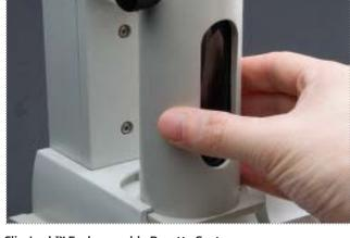
**Clip-Lock™ Exchangeable Burette System**With Clip-Lock™, it only takes a few seconds to exchange the reagent burettes to perform a different titration
