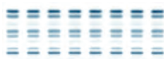
Merck Millipore TLC plates deliver highly reproducible sharp bands over the whole plate as demonstrated by the parallel separation of a lipophilic dye mixture on a silica gel 60 classical TLC plate
