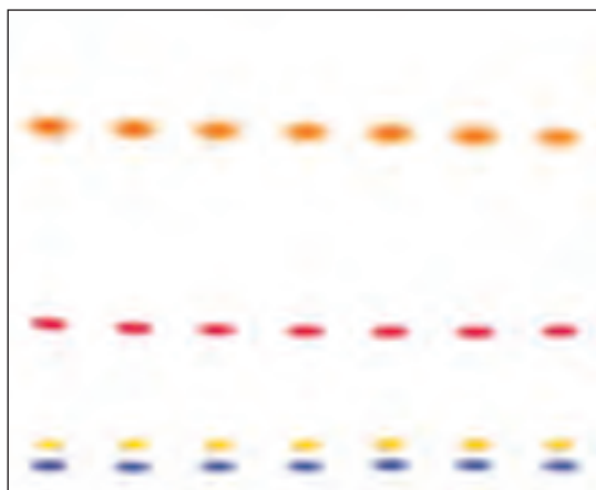
The chromatogram shows four clearly separated spots under Ph Eur test conditions and fulfils Ph Eur requirements (see R_f values).
